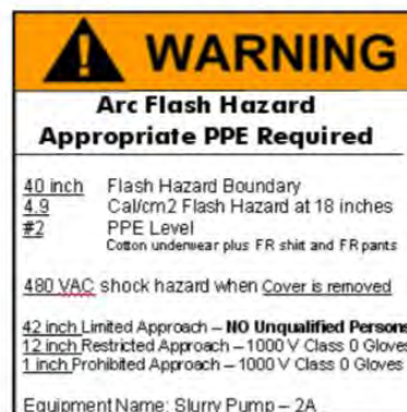
Detailed (preferred) arc flash label example
