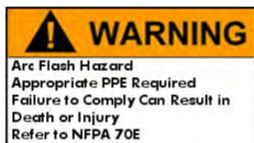
Minimum arc flash label example
