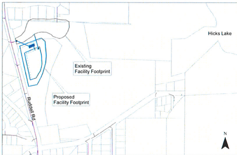
Figure 1. Layout of Proposed Infiltration Facility
