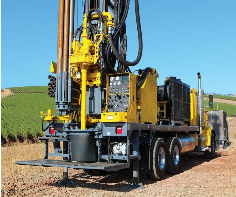
Typical Well Rotary Drilling Rig (0 to 460 ft deep)
