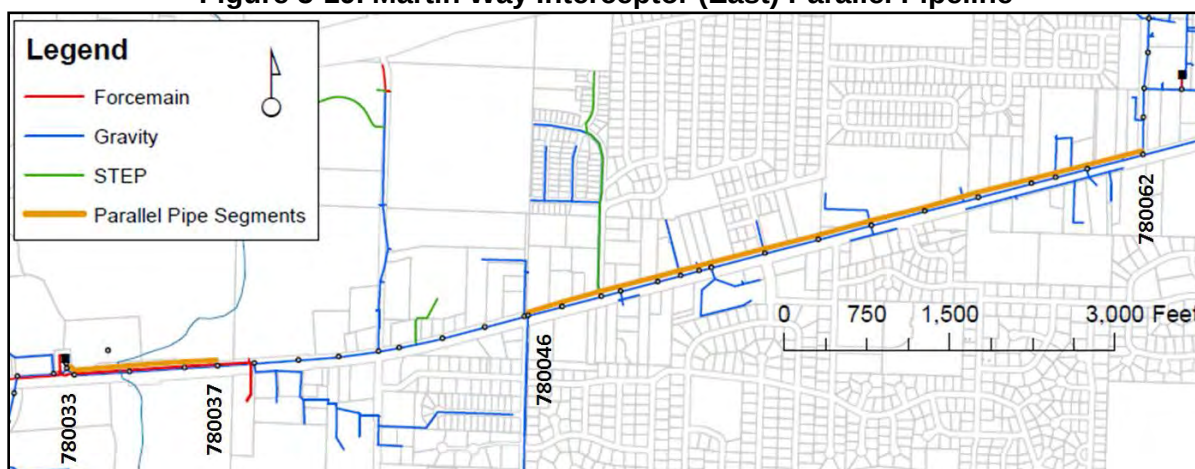
Figure 5-19. Martin Way Interceptor (East) Parallel Pipeline
